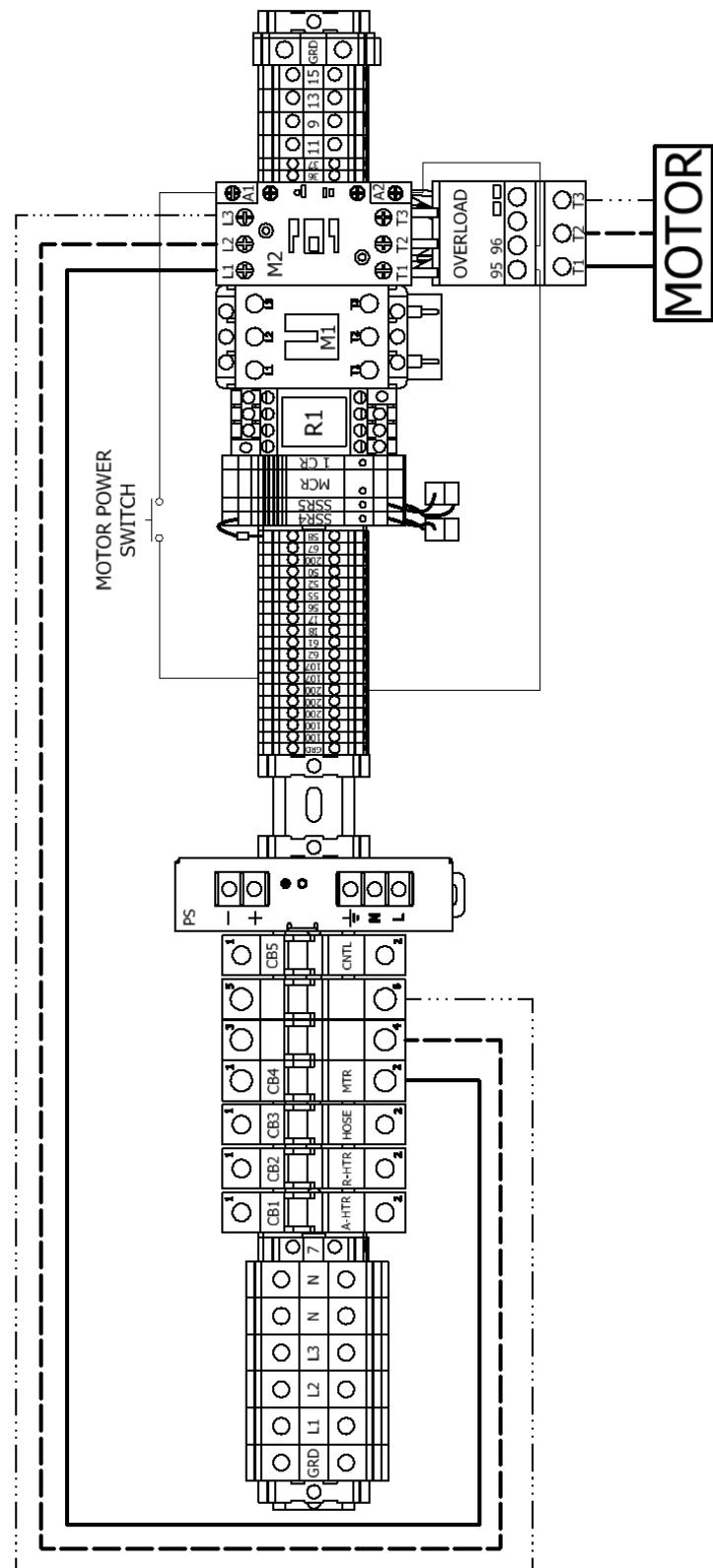
Point to Point Diagrams (ALL CONSOLES)24 VDC Power Circuit
