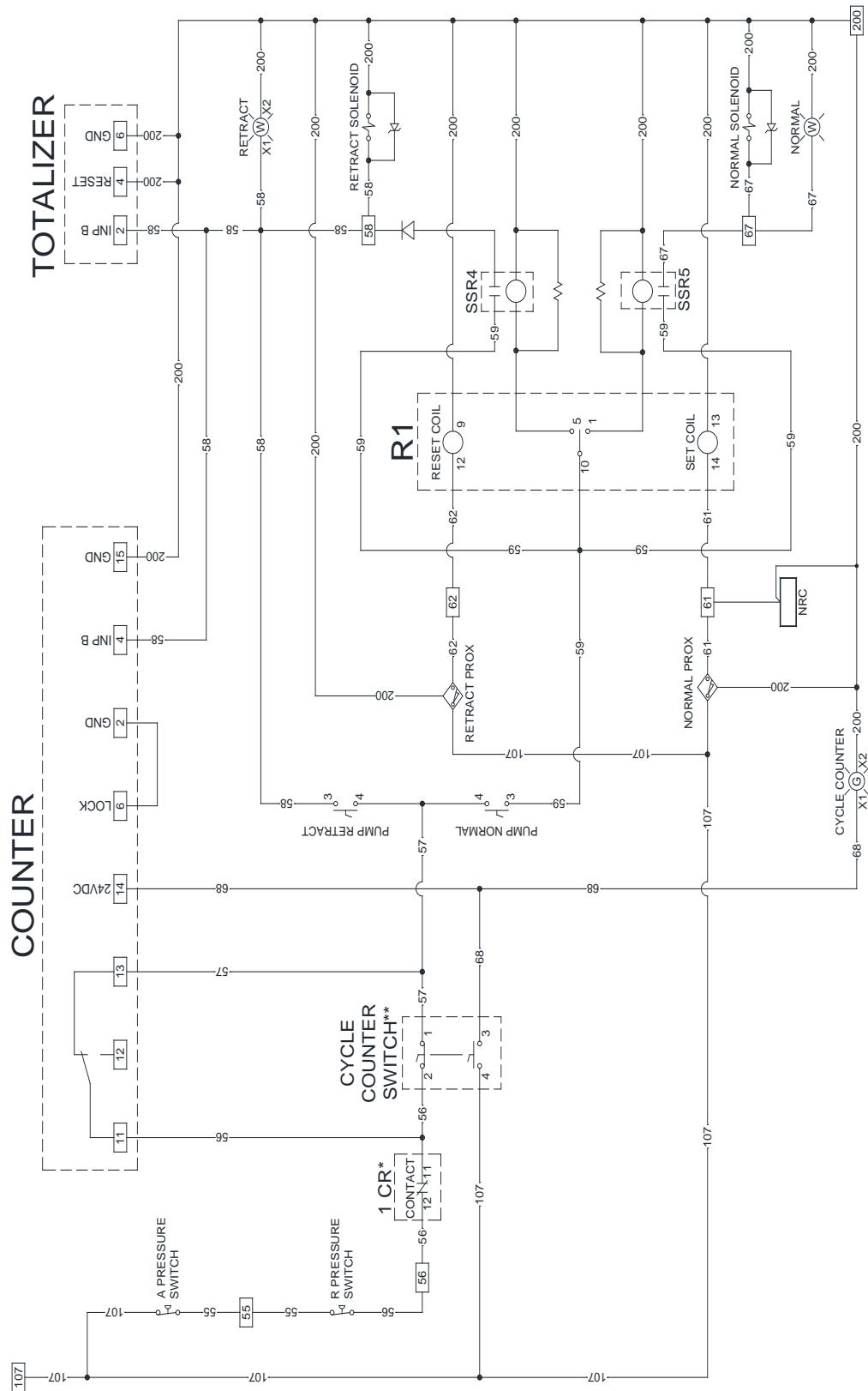
\*See Pressure Balance Control Circuit (Pg. 40) for complete 1 CR wire connections
